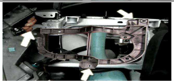
After installing the mounting bracket for both side, put the front bumper back on the car. Bolt all the screws back on the bumper.
