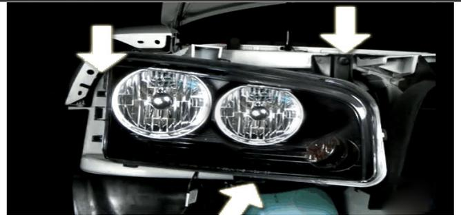
Install the Mounting Bracket first onto the car, align the screws where you mount the OEM Headlights. (as shown)
