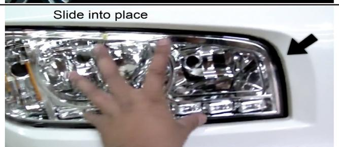
Once you align the screw to the mounting bracket, bolt the screws back on using a 10mm socket. There are four mounting point behind the headlight.
