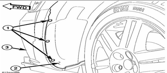
Once you remove the wheel cover, there are two screws on the each side of the bumper (side bumper).
