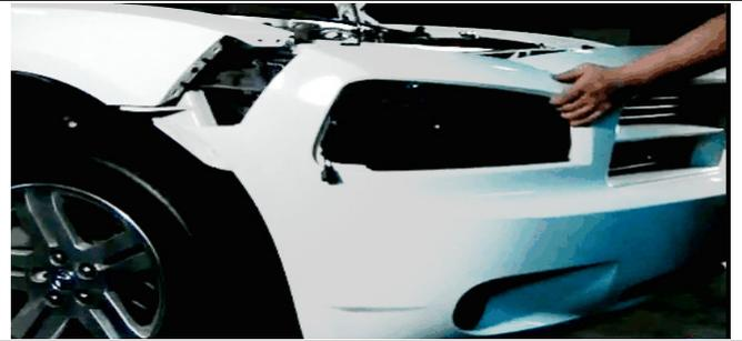
Remove the headlight assembly from the vehicle. There are three screws, two on the top, and one on the bottom of the headlight.
