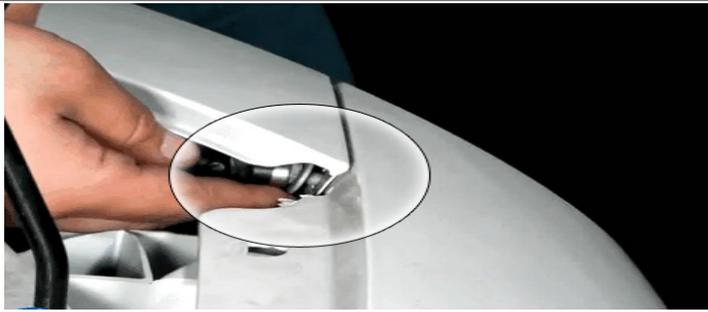
Remove the nine screws that secure the belly pan to the underbody using a 7mm socket.
