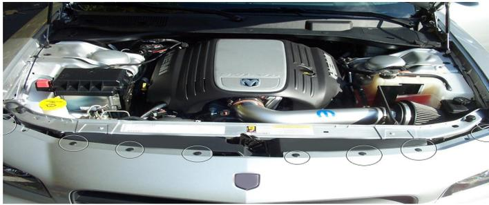
Remove the Screw that is holding the Fender, using a 10mm socket. On both ends
